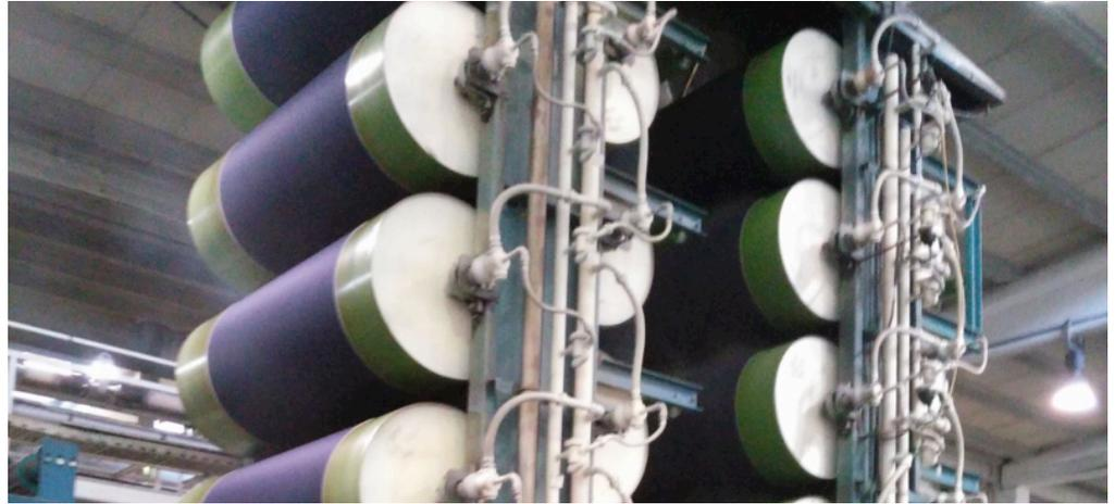
When a denim manufacturing company contacted energy efficiency expert, Kolorgen Ltd., they had an interesting challenge. They'd never been able to insulate their rotating drying cans to save energy. This was due to the limited amount of space and the constant rotation during the manufacturing process.
