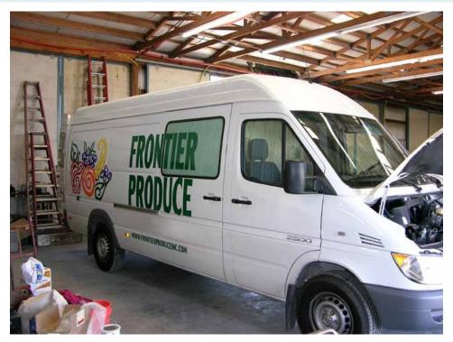
Frontier Produce in Tulsa, Oklahoma wanted to reduce the fuel used to cool the back of their delivery van and increase gas mileage of their vehicle. Energy Protect<sup>™</sup> was used to insulate the interior walls and ceiling of the van to reduce heat gain and make the vehicle more fuel efficient.
