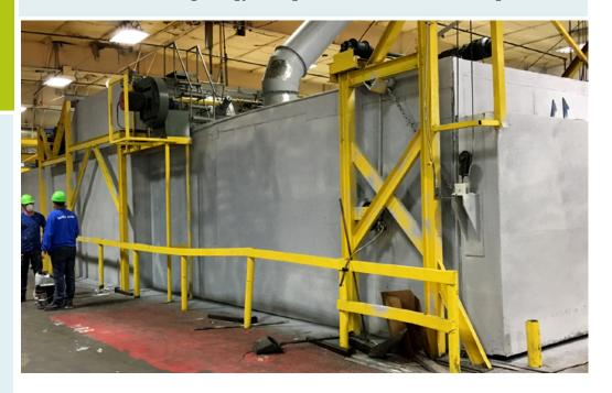
One of the industrial applications that the Heat Shield™ EPX-H2O thermal insulation coating was specifically designed for is the insulation of large industrial ovens to solve issues with energy loss and personnel safety without interfering with the oven related processes.
