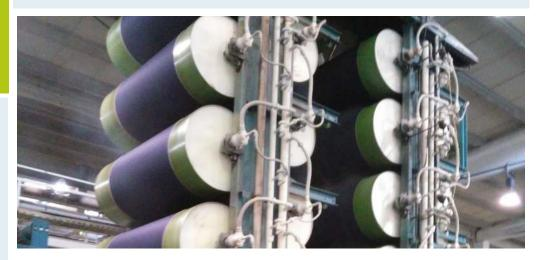
When a denim manufacturing company contacted energy efficiency expert, Kolorgen Ltd., they had an interesting challenge. They'd never been able to insulate their rotating drying cans to save energy. This was due to the limited amount of space and the constant rotation during the manufacturing process.
