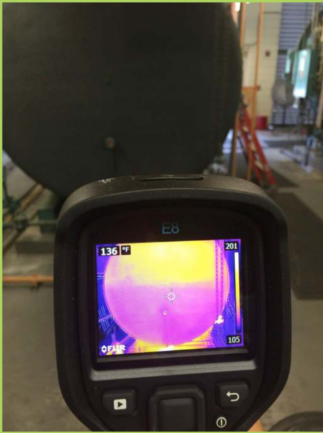
Infrared imaging during application. Top half of boiler had 4-coats and bottom half had 6-coats of Heat Shield EPX-H20. The temperature was reduced below safe touch to 136F.
