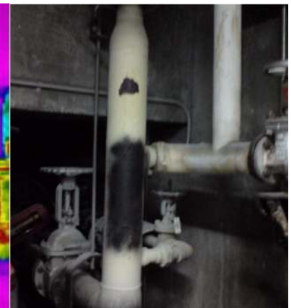
The measurement area was painted black to avoid any mis-reading by the thermal imaging equipment.
