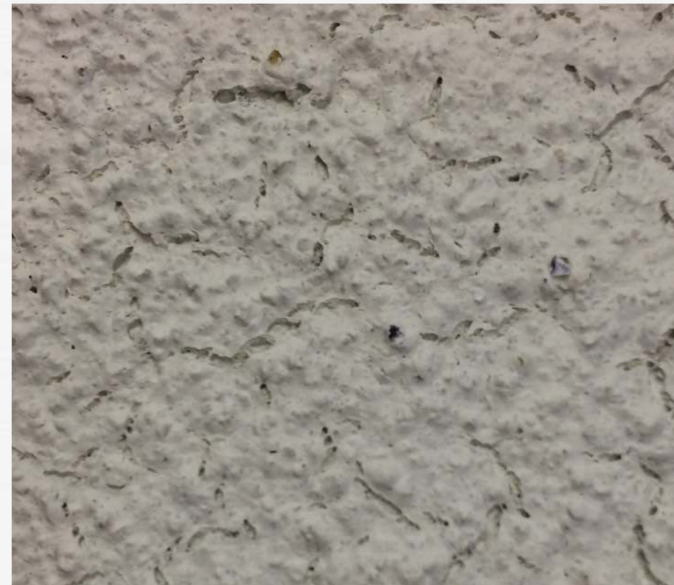
Example of hairline cracks on film when applied past 24 hr pot life.
