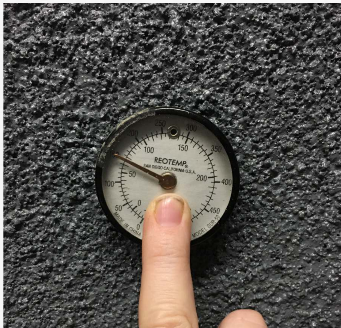
Surface contact, magnetic thermometer. Allowed to come to a steady state temperature for 20 minutes.
