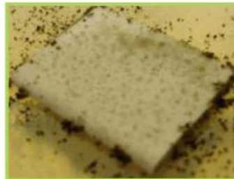
Uncoated panel: Covered with mold growth.
